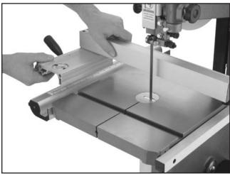
Figure 18. Installing fence onto rails.
